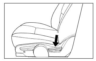
To recline the seatback on the driver's seat, lift the lever on the rear outboard side of the seat and move the seatback to the desired position. Then release the lever to lock the seatback in place.
